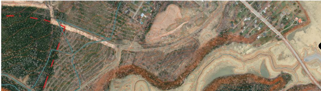
Step Five (Figure 6.0) - Observations from the drone footage and base imagery are mapped into polygons on the base map.
