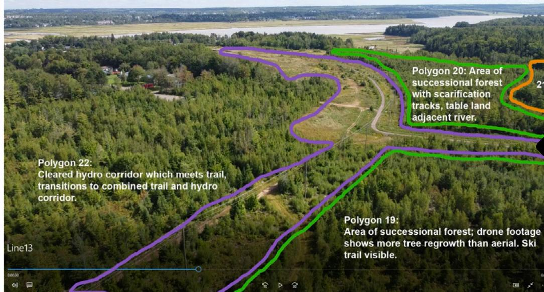
Step Four (Figure 5.0) - Example of Noted Features Visible on Drone Footage.
