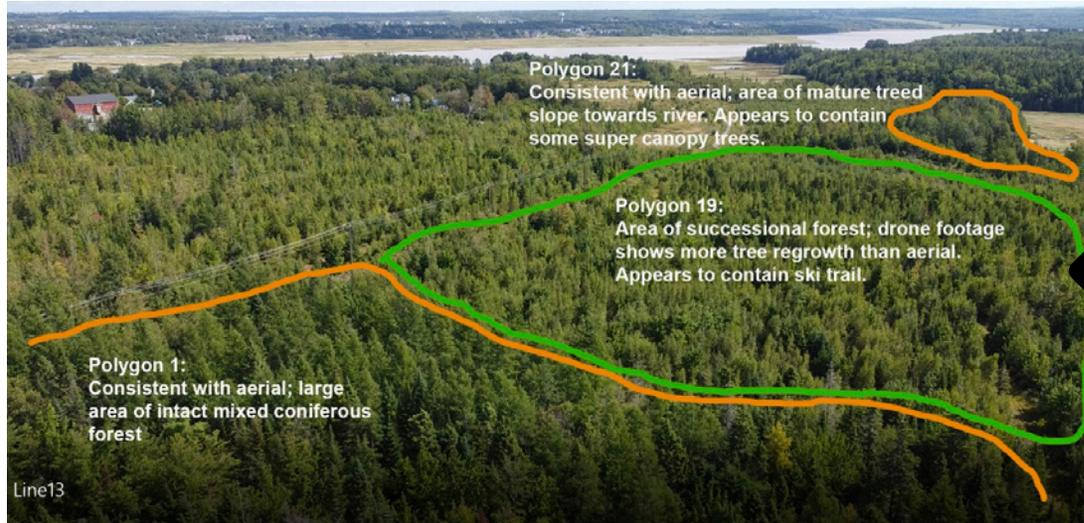
Step Three (Figure 4.0) - Direct observation and categorization of land characteristics is made by viewing drone footage, cross-referenced with other available data.
