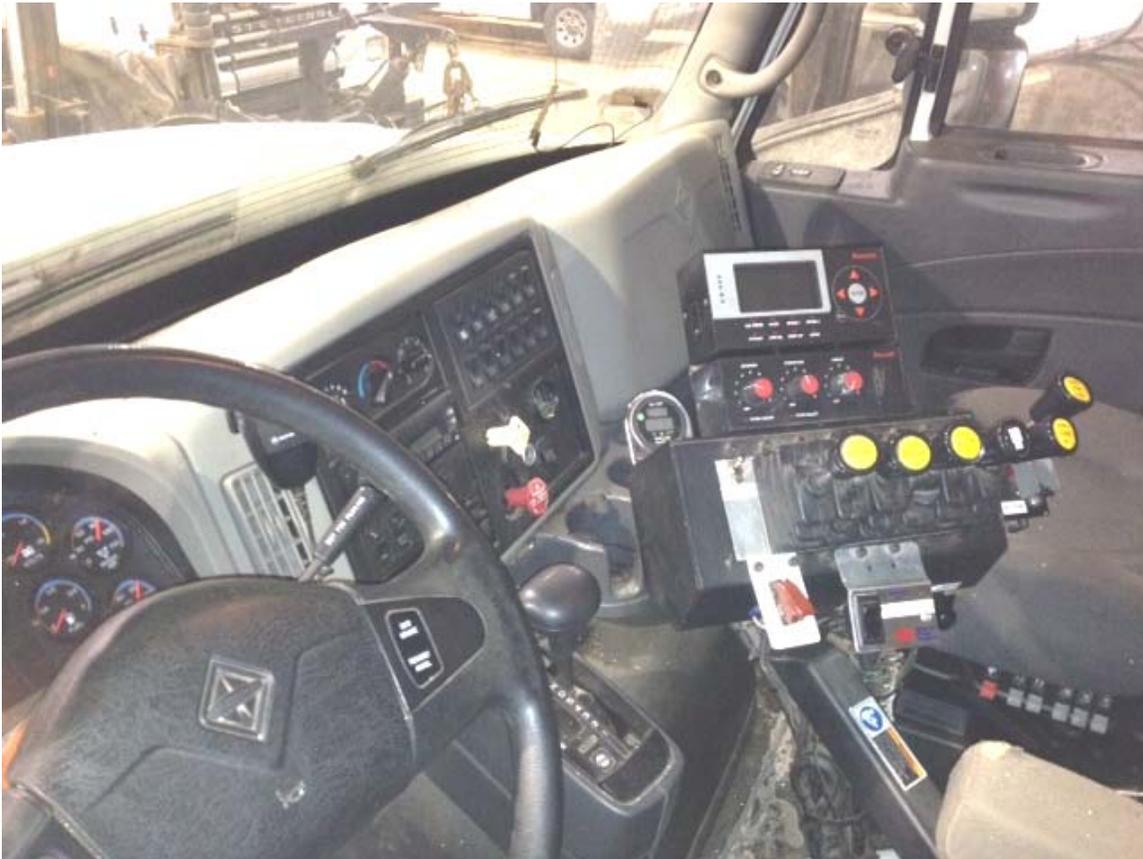
**Picture 1 – 420 Compu-spread regulators**
