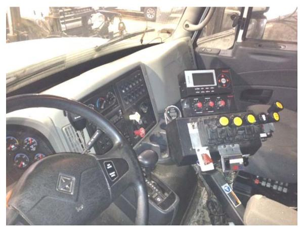
Picture 1 – 420 Compu-spread regulators
