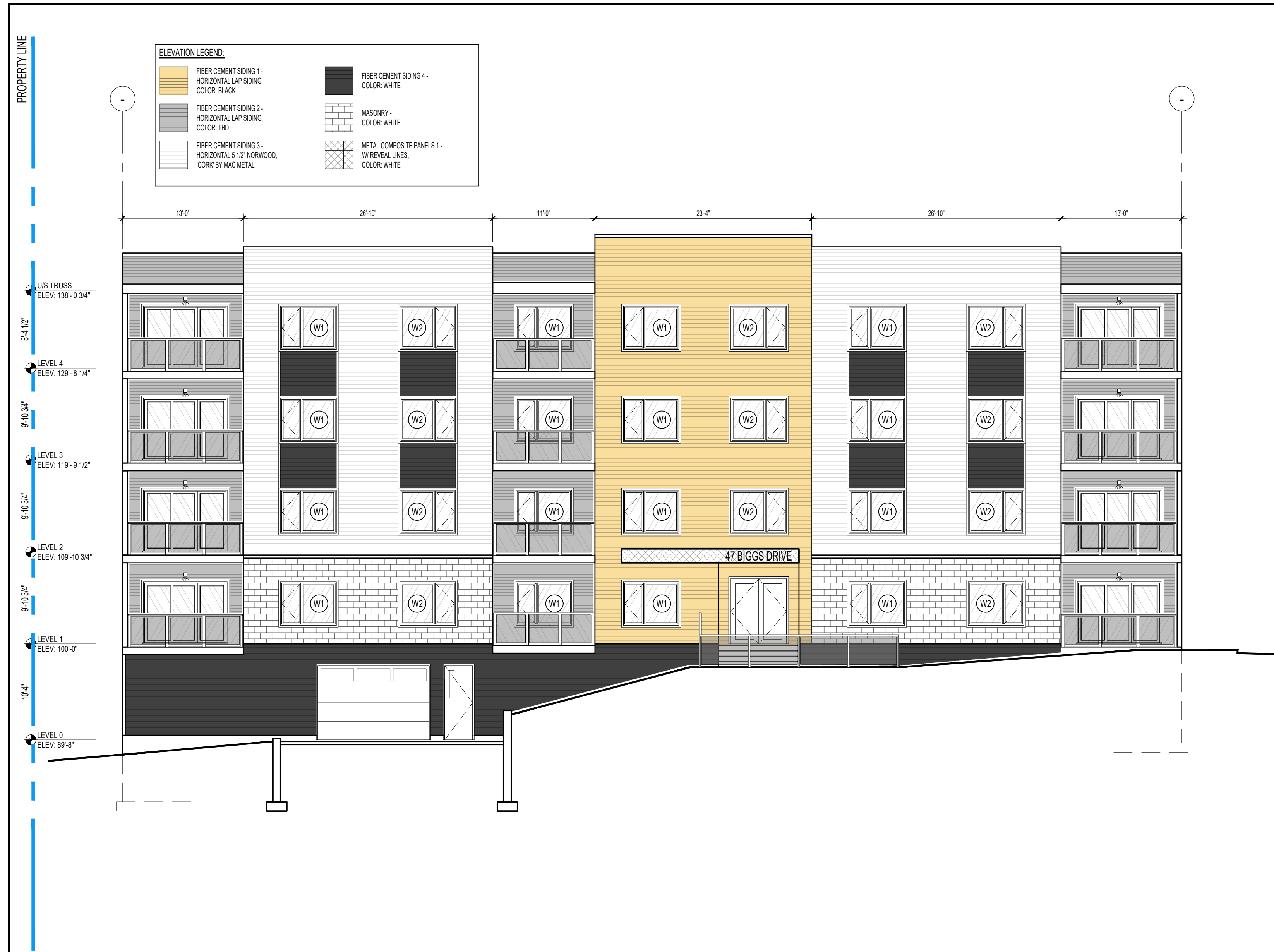
① ELEVATION - WEST (BIGGS DRIVE) SCALE: 1/8"=1'-0"
